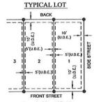
ALL UTILITY AND DRAINAGE WAY EASEMENTS ARE 10' IN WIDTH ALONG STREET FRONTAGE AND REAR LOT LINES, (EXCEPT ALONG WALL AVENUE RICHT OF WAY), AND 5' ON EACH SIDE OF SIDE LOT LINES, UNLESS OTHERWISE NOTED.
